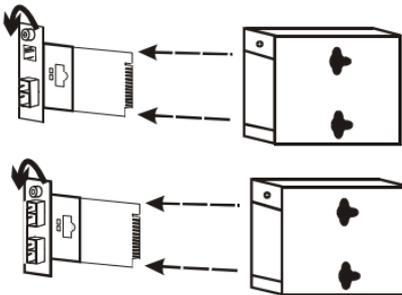
Unscrew the hand screw counter clockwise by using hand or screwdriver and pull the media converter module out on the carrier
