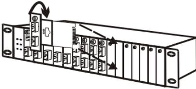
Insert the media converter module into an available slot and fasten the hand screw clockwise by using hand or screwdriver.
